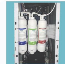
Photo D 4. Remove and replace filters in the same sequence
