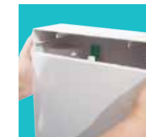
Photo D 4. Lift up the cover
