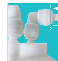
Photo G Use your finger to push in the ring as shown in direction (1) and hold it while you pull out the tube as shown in direction (2)
